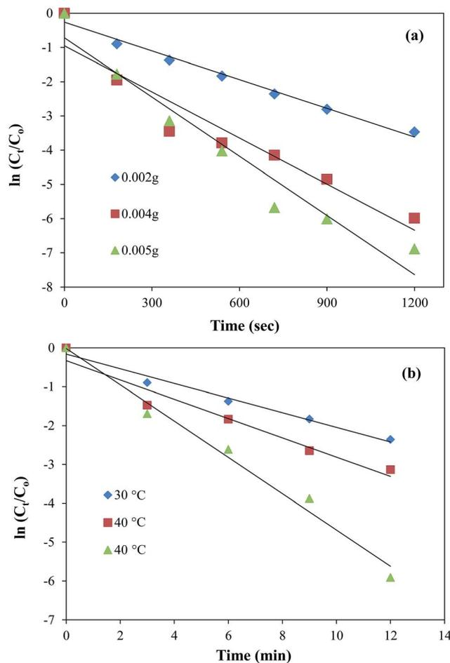
Fig. 8 Dependence of  $k_{\text{app}}$  on (a) the amount of catalyst at 30 °C and (b) temperature. Reaction conditions; 0.5 mM aqueous solution of 2-nitroaniline = 50 ml,  $\text{NaBH}_4 = 0.1$  g, graphene oxide-gold catalyst = 5 mg, 100 rpm.
