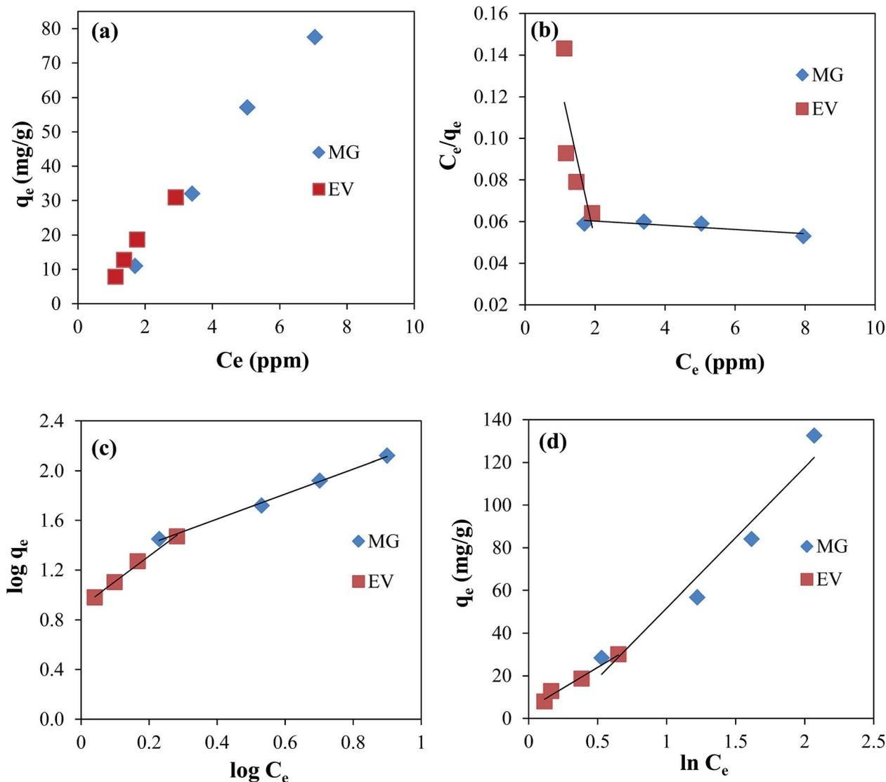
Fig. 4 Plots of (a)  $q_e$  versus  $C_e$ , (b) Langmuir isotherm, (c) Freundlich isotherm, and (d) Temkin isotherm for the adsorption of MG and EV dyes on GO-Au nanocomposite. Reaction conditions; adsorbent = 0.005 g, concentration of dyes solution = 3, 5, 7, and 10  $\mu$ M volume of dyes solution = 50 ml, 100 rpm, 25  $^{\circ}$ C.
