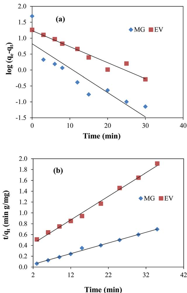
Fig. 5 Plots of (a) pseudo first-order kinetic model, (b) pseudo second-order kinetic model for malachite green (MG) and ethyl violet (EV) adsorption. Reaction conditions; 7  $\mu\text{M}$  solution of each dye = 50 ml, 100 rpm, 30  $^\circ\text{C}$ .
