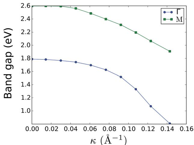
Fig. 6 Electronic band gap at the  $\Gamma$  and  $M$  points as a function of curvature. The system band gap is always located at  $\Gamma$ ; the band gap at  $M$  is just a parameter to quantify bending effects. Surface states were ignored in the gap measurement.
