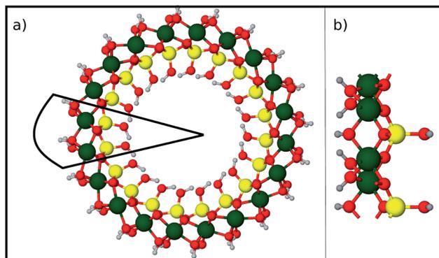
Fig. 7 Structure of an imogolite nanotube. (a) An axial view of imogolite for  $N_\theta = 10$ . The basic unit is marked by the continuous black line. (b) A side view of the basic imogolite unit  $[(\text{OH})_3\text{Al}_2\text{O}_3\text{SiOH}]_2$ , that is repeated  $N_\theta$  times to form the nanotube. Green Al; red O; yellow Si; and light gray H.
