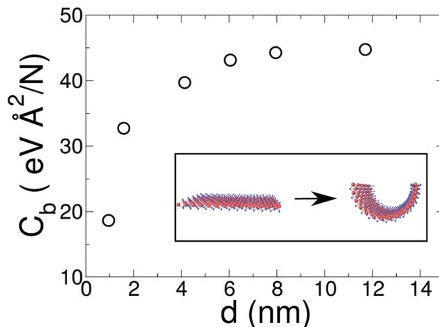
Fig. 4 Bending modulus of a MoS<sub>2</sub> ribbon as a function of its width  $d$ . MO: blue; S: red.
