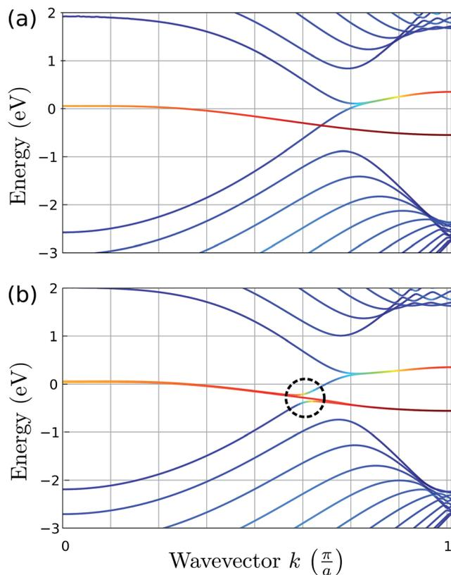
Fig. 3 Band structure of a flat GNR (a) and a bent GNR, with the curvature radius  $R = 0.5$  nm (b). The reddish bands are derived from the edges of the ribbon, the blue bands do not have a projection on the edges and intermediate colors apply for mixed states.
