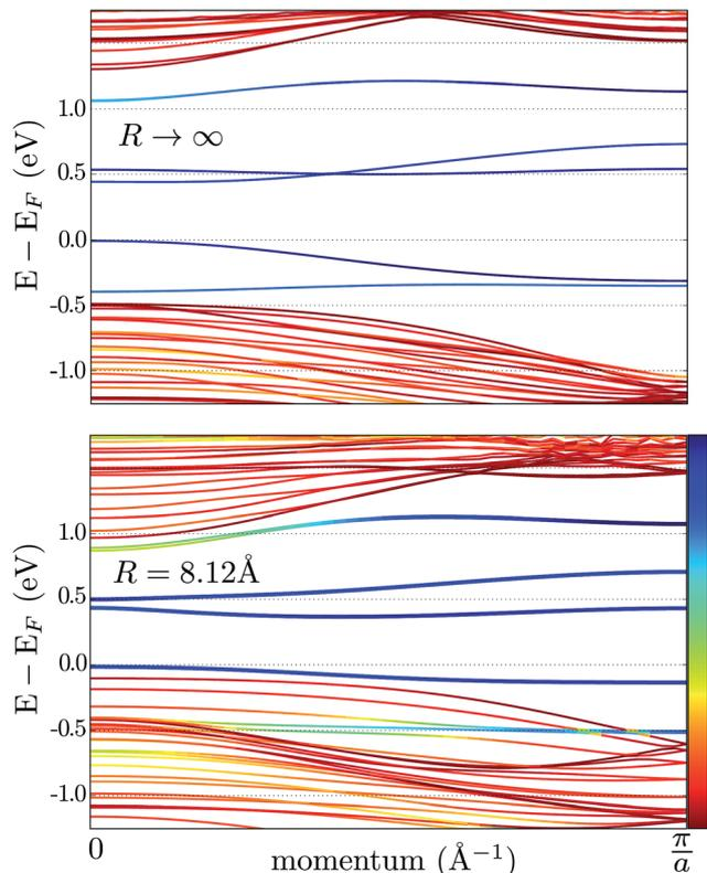
Fig. 5 Band structure of an armchair MoS<sub>2</sub> nanoribbon. The upper and lower panels correspond to a flat ( $R \rightarrow \infty$ ) and a bent nanoribbon, respectively. The color code shows the (real-space) localization of the eigenvalues: red is used for the inner subbands (i.e. bulk-like), while the edge subbands are blue; intermediate colors correspond to the hybridization of bulk and edge states.
