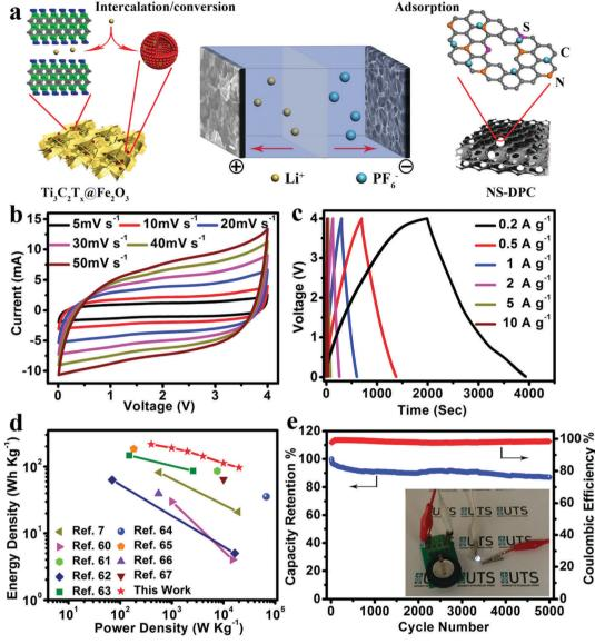
Fig. 5 (a) Schematic illustration of the charge-storage mechanisms for the  $Ti_3C_2T_x@Fe_2O_3//NS-DPC$  LIC device. (b) CV curves and (c) charge-discharge curves of the  $Ti_3C_2T_x@Fe_2O_3//NS-DPC$  LIC device and other previously reported devices. (e) Cycling stability of the  $Ti_3C_2T_x@Fe_2O_3//NS-DPC$  device at a current density of 5 A  $g^{-1}$ ; the inset is a demonstration of the LIC device powering an LED.
