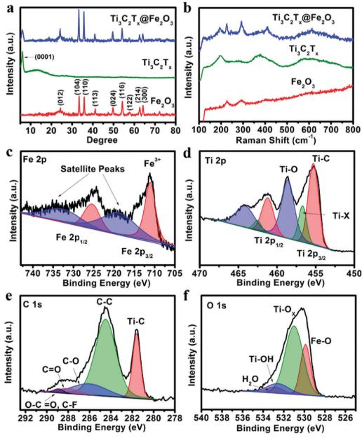
Fig. 1 (a) XRD patterns and (b) Raman spectra of the  $Fe_2O_3$ ,  $Ti_3C_2T_x$  and  $Ti_3C_2T_x$ @ $Fe_2O_3$  samples. (c) Fe 2p, (d) Ti 2p, (e) C 1s, and (f) O 1s XPS spectra of the  $Ti_3C_2T_x$ @  $Fe_2O_3$  nanocomposite.
