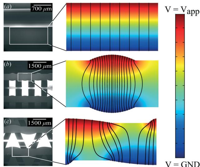
Fig. 3 Modeled potential distribution and electric field lines inside the microfluidic channels, (a) for homogeneous hydrogels, (b) for rectangular heterogeneous hydrogels and (c) for trapezoidal heterogeneous hydrogels.
