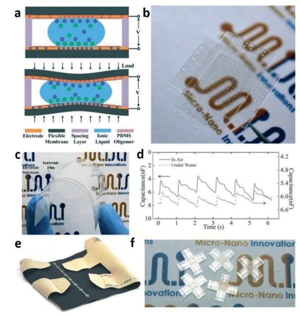
**Fig. 10** (a) lontronic droplet sensor operation principle. (b) Photo of an iontronic microdroplet sensing array. (c) Photo of a flexible ionic gel film on an electrode substrate. (d) Real-time pulse pressure waveforms in dry and underwater environments. (e) Photo of a commercial inelastic legging integrated with the iontronic flexible sensing array. (f) Prototypes of microfluidic tactile sensors for three-dimensional force measurements.
