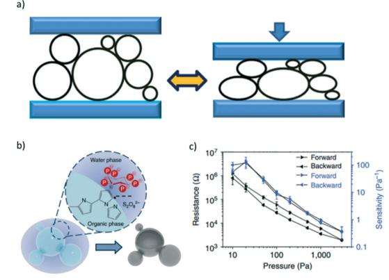
**Fig. 8** a) Schematic illustration of the elasticity of hollow sphere structured polypyrrole (PPy). b) Schematic illustration of the phase separation between water and organic components for the synthesis of PPy hydrogels. c) Electrical resistance response to induced pressure.<sup>84</sup>
