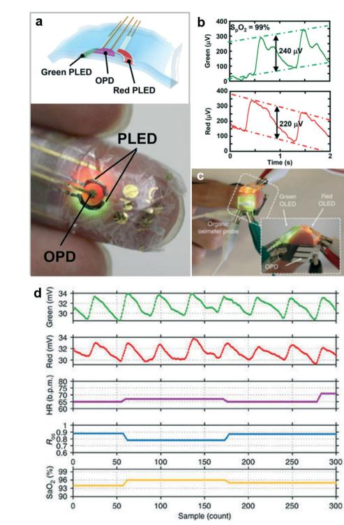
Fig. 14 Reflectance based layout and application picture of the pulse oximeter system with concentric LED's and circular photodiode scheme (a), with resulting signal output (b). Organic transmission based oximeter (c) with resulting raw data and signal extraction (d).
