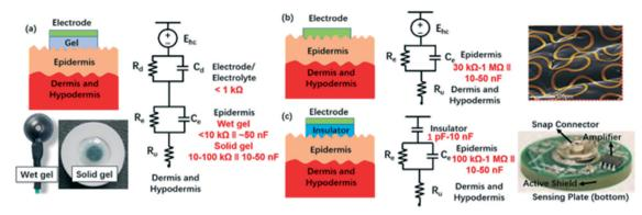
**Fig. 3** Equivalent circuit models of electrode-skin interfaces for different electrode designs. (a) Gel electrodes, including wet and solid forms (disposable deep EEG cup electrode, Rhythmlink; ECG electrode H1354LG, Kendall). (b) Dry contact electrodes.<sup>61</sup> (c) Dry capacitive (non-contact) electrodes.<sup>51</sup>
