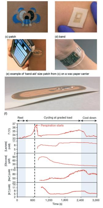
**Fig. 17** Bringing electrochemical sensors directly onto skin to detect sweat (adapted).<sup>158</sup> In all the examples provided in the figure, technology is mechanically compliant to skin, which is a first step to reduce the sweat volume between skin and sensors. The data shown in (f) is for a human subject wearing the technology shown in (d).<sup>178</sup>
