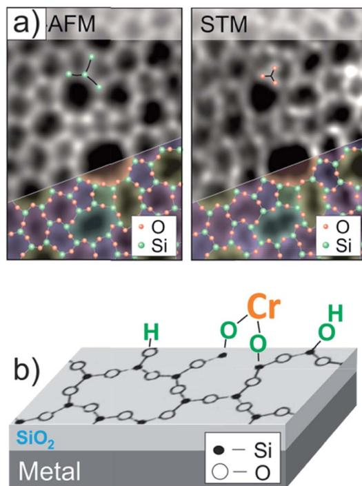
**Fig. 1** (a) Atomic force microscope (AFM) and STM images of the amorphous bilayer silica film grown on Ru(0001), that are superimposed with a silica network. (b) Schematic view of a planar model system for the Phillips catalyst, where Cr species are anchored onto an atomically flat hydroxylated silicate film (reprinted with permission from ref. 43. Copyright (2017) Elsevier).
