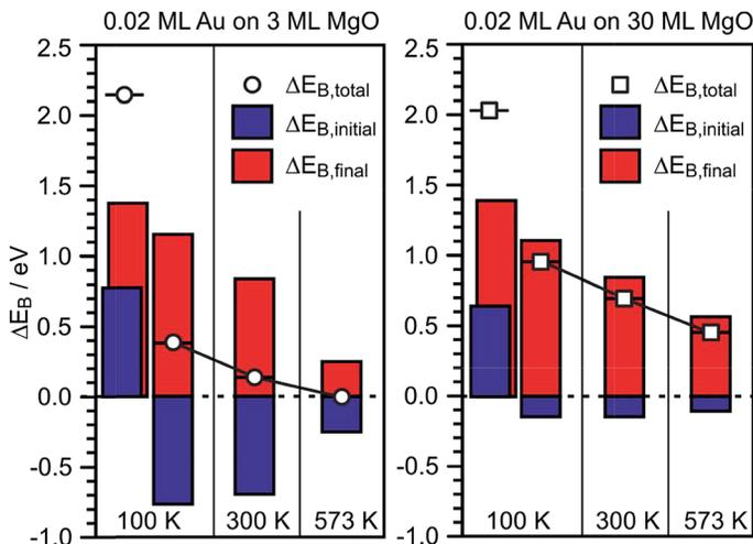
Fig. 8 Graphical representation of the  $E_B$ -shifts derived from  $\Delta\beta$  measurements for 0.02 ML Au on 3 ML MgO(001)/Ag(001) (left) and 0.2 ML Au on 30 ML MgO(001)/Ag(001) (right) with reference to Au(111) from Table 1.
