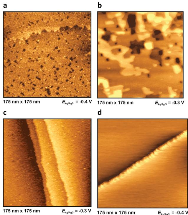
Fig. 4 *In situ* STM images in BMIPF<sub>6</sub> at  $-0.3$  V or  $-0.4$  V for Au(100) (a), Ag(100) (b), Pt(100) (c) and HOPG (d). The images were taken about 30 minutes after assembling the cell.
