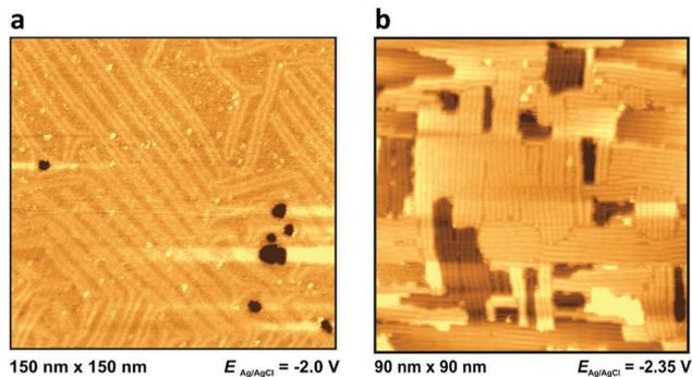
Fig. 7 Metal surface at extreme negative potentials: reconstructed Au(111) in PMPiTf<sub>2</sub>N (a) and Au(100) BMITf<sub>2</sub>N (b) surfaces, at potentials indicated. For other images of the reconstruction lines see Fig. 8d of ref. 34, Fig. 4c and 5b of ref. 35, as well as Fig. 10c and 10d of ref. 36.
