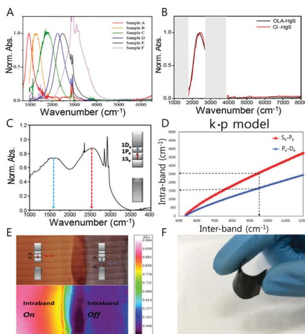
Fig. 5 (A) Absorption spectra of HgS CQD (B) HgS absorption with oleylamine and atomic ligand (C)  $1S_e-1P_e$  and  $1P_e-1D_e$  absorption spectrum (D) intraband and bandgap correlation-based k-p model (E) IR microscope image of doping controlled HgS permission from ref. 24. Copyright 2016 American Chemical Society. (F) Flexible HgSe CQD film.
