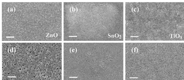
Fig. 3 SEM images of perovskite films deposited on ZnO, SnO<sub>2</sub> and TiO<sub>x</sub> substrates before (a–c) and after (d–f) vacuum-processing, respectively. The scale bar is 1  $\mu\text{m}$ .
