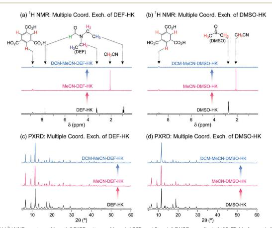
Fig. 14 (a and b) <sup>1</sup>H NMR spectra and (c and d) PXRD patterns of (a and c) DEF- and (b and d) DMSO-coordinated HKUST-1 before and after initial MeCN treatment and subsequent DCM treatment. NMR spectra were measured after the powder samples were completely dissolved in D2SO4. Reprinted (adapted) with permission from ref. 69. Copyright (2017) American Chemical Society.
