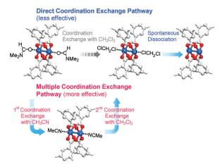
Fig. 8 Schematics illustrating direct and multiple coordination exchange pathways for the activation of the paddle wheel-like (Cu<sup>II</sup>)<sub>2</sub> node of HKUST-1. Hydrogen atoms bound to the carbon atoms in the benzene moieties are omitted for clarity. Reprinted (adapted) with permission from ref. 69. Copyright (2017) American Chemical Society.
