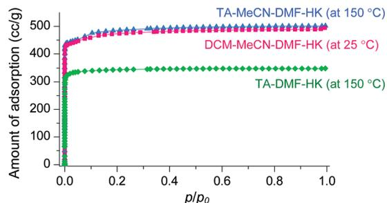
Fig. 13  $N_2$  adsorption isotherms of TA-DMF-HK (green), TA-MeCN-DMF-HK (blue), and DCM-MeCN-DMF-HK (pink). Reprinted (adapted) with permission from ref. 69. Copyright (2017) American Chemical Society.
