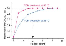
Fig. 6 Changes in the amount of MeOH dissociated from MeOH-HK with respect to the number of TCM treatments performed at 25  $^{\circ}$ C (blue) and 55  $^{\circ}$ C (red). Reprinted (adapted) with permission from ref. 70. Copyright (2018) American Chemical Society.
