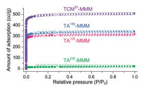
Fig. 19  $N_2$  adsorption/desorption isotherms of  $TA^{105}$ -,  $TA^{150}$ -,  $TA^{200}$ -, and TCM<sup>25</sup>-MMM. The isotherms for the TCM<sup>25</sup>-MMM sample were measured after applying vacuum at room temperature for 4 h. Reprinted (adapted) with permission from ref. 70. Copyright (2018) American Chemical Society.
