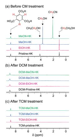
Fig. 4 <sup>1</sup>H NMR spectra of pristine-, EtOH-, MeOH-, and MeCN-coordinated HKUST-1 (a) before chloromethane treatment, (b) after DCM treatment, and (c) after TCM treatment. NMR spectra were measured after completely dissolving the powder samples in D<sub>2</sub>SO<sub>4</sub>. Reprinted (adapted) with permission from ref. 68 and 70. Copyright (2015 and 2018) American Chemical Society.
