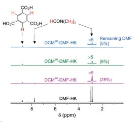
**Fig. 7** <sup>1</sup>H NMR spectra of DMF-coordinated HKUST-1 before and after DCM treatment 10, 20, and 30 times. NMR spectra were measured after the powder samples were completely dissolved in D<sub>2</sub>SO<sub>4</sub>. Reprinted (adapted) with permission from ref. 69. Copyright (2017) American Chemical Society.
