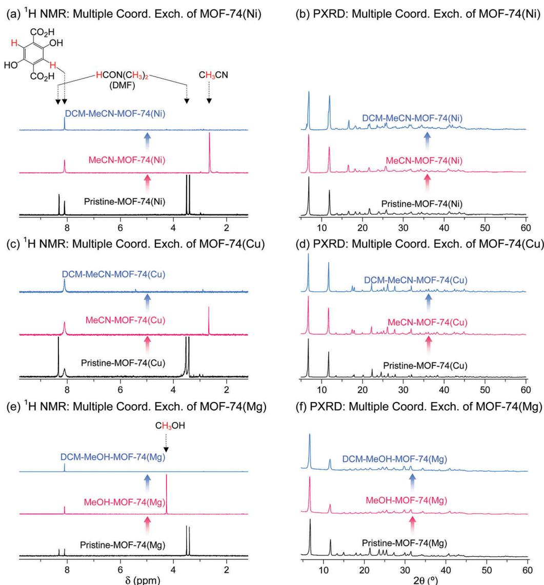
Fig. 15 (a, c and e)  $^1\text{H}$  NMR spectra and (b, d and f) PXRD patterns of DMF-coordinated (a and b) MOF-74(Ni), (c and d) MOF-74(Cu), and (e and f) MOF-74(Mg) before and after initial (a–d) MeCN and (e and f) MeOH treatment and subsequent DCM treatment. NMR spectra were measured after the powder samples were completely dissolved in  $\text{D}_2\text{SO}_4$ . Reprinted (adapted) with permission from ref. 69. Copyright (2017) American Chemical Society.
