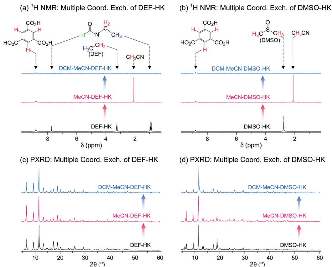
Fig. 14 (a and b)  $^1\text{H}$  NMR spectra and (c and d) PXRD patterns of (a and c) DEF- and (b and d) DMSO-coordinated HKUST-1 before and after initial MeCN treatment and subsequent DCM treatment. NMR spectra were measured after the powder samples were completely dissolved in  $\text{D}_2\text{SO}_4$ . Reprinted (adapted) with permission from ref. 69. Copyright (2017) American Chemical Society.
