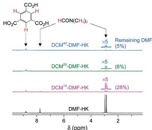
Fig. 7  $^1\text{H}$  NMR spectra of DMF-coordinated HKUST-1 before and after DCM treatment 10, 20, and 30 times. NMR spectra were measured after the powder samples were completely dissolved in  $\text{D}_2\text{SO}_4$ . Reprinted (adapted) with permission from ref. 69. Copyright (2017) American Chemical Society.
