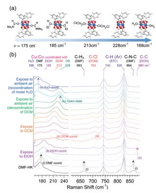
Fig. 11 (a) Illustrations of DMF-coordinated, EtOH-coordinated, DCMcoordinated, open-state, and H<sub>2</sub>O-coordinated (Cu<sup>II</sup>)<sub>2</sub> centers in HKUST-1 (from left to right). (b) Successive changes of the in situ Raman spectra of DMF-coordinated HKUST-1 during sequential exposure to EtOH, DCM, and ambient air. Reprinted (adapted) with permission from ref. 69. Copyright (2017) American Chemical Society.
