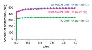
Fig. 13 N<sub>2</sub> adsorption isotherms of TA-DMF-HK (green), TA-MeCN-DMF-HK (blue), and DCM-MeCN-DMF-HK (pink), Reprinted (adapted) with permission from ref. 69. Copyright (2017) American Chemical Society
