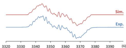
**Fig. 2** Experimental (bottom) and simulated (top) EPR spectra of **2** ( $g = 2.0107$ ; hyperfine coupling constants:  $a(^{14}N) = 23.4, 9.1, 6.9$  MHz,  $a(^{11}B) = 6.7$  MHz,  $a(^1H) = 5.3, 3.6$  MHz,  $a(^{19}F) = 2.6, 1.7$  MHz).
