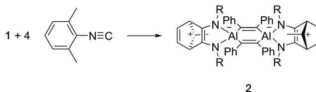
Scheme 2 Reaction of 2,6-dimethylphenylisonitrile with **1**.
