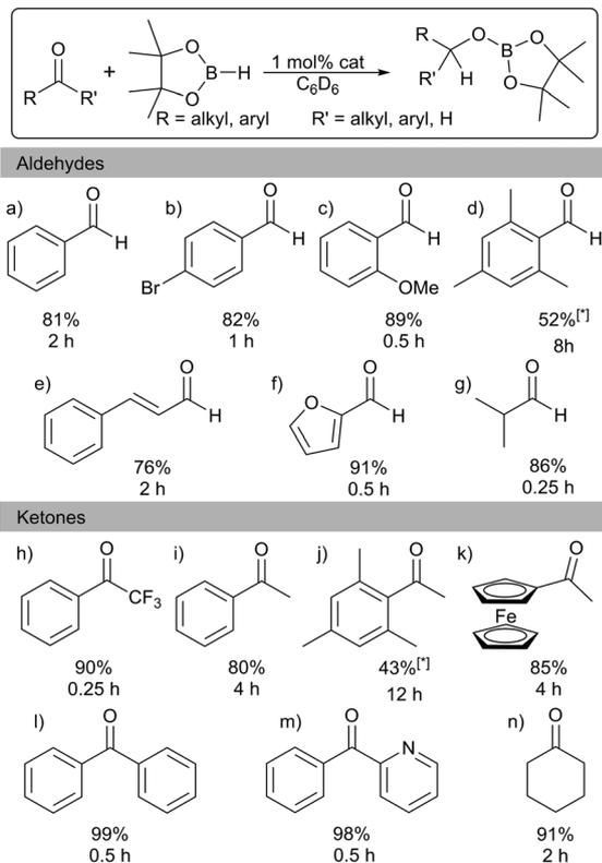
Catalysis performed in C<sub>6</sub>D<sub>6</sub>, at room temperature, 1 mol% pre-catalyst. <sup>1</sup>H NMR yields relative to internal standard hexamethylcyclotrisiloxane. [\*] heated to 70 °C.
