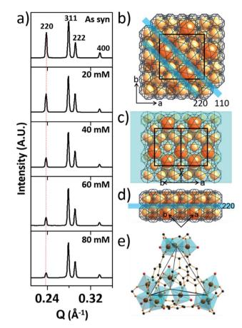
Fig. 2 (a) SAXS spectra of the pristine MIL-100(Fe) and MIL-100(Fe)-20, 40, 60 and 80. (b) The unit cell of MIL-100(Fe) with the (110) and (220) lattice planes (blue colored) and (c and d) front (cross section) and side views of the (220) lattice plane. (e) Structure of the tetrahedral secondary building unit (SBU) of MIL-100(Fe).
