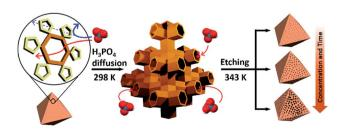
Scheme 1 Illustration of the etching process for MIL-100(Fe). Left: MIL-100(Fe) crystal with hexagonal and pentagonal windows; middle: acid diffusion into tetrahedral channels through hexagonal windows; right: resulting mesopores after etching.
