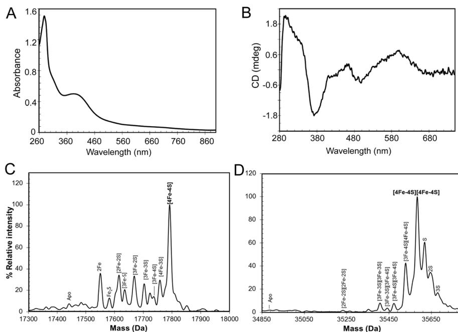
Fig. 2 Characterization of the RirA iron-sulfur cluster. (A) UV-visible absorbance and (B) CD spectra of reconstituted RirA (371  $\mu$ M [4Fe-4S] RirA) in buffer B. Pathlength 1 mm. (C) and (D) Positive ion mode ESI-MS deconvoluted spectra of RirA (30  $\mu$ M in cluster in 250 mM ammonium acetate pH 7.32) under non-denaturing conditions in the monomer (C) and dimer (D) mass regions.
