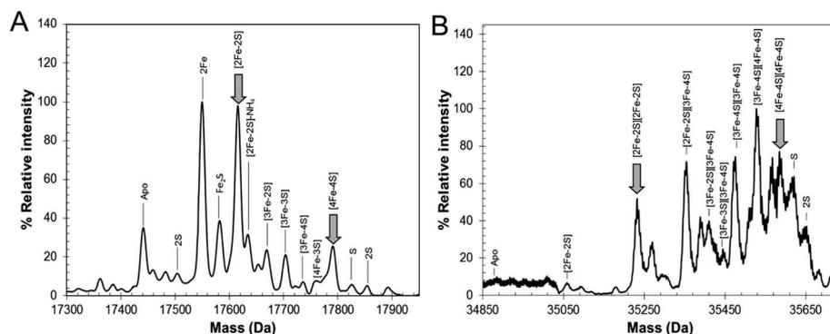
Fig. 5 ESI-MS analysis of RirA following low iron-mediated cluster conversion. Positive ion mode ESI-TOF native mass spectra of  $\sim 21 \mu\text{M}$  [4Fe-4S] RirA in 250 mM ammonium acetate pH 7.35 following treatment with 1 mM EDTA for 2.5 h. Deconvoluted spectrum in the (A) monomer and (B) dimer mass regions. ESI-MS data for RirA prior to the addition of EDTA are shown in Fig. 3.
