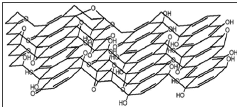
Fig. 21 Structure model of GO. Reproduced with permission.<sup>249</sup> © 2006 American Chemical Society.
