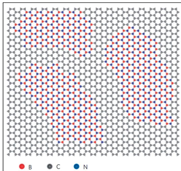
Fig. 25 Atomic model of h-BNC film showing hybridized h-BN and graphene domains. Reproduced with permission.<sup>279</sup> © 2010 Nature Publishing Group.
