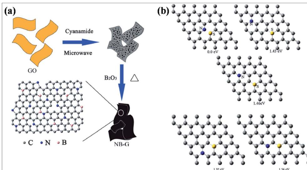
Fig. 27 (a) Fabrication of the NB-G framework from GO. Reproduced with permission.<sup>287</sup> © 2013 Royal Society of Chemistry. (b) Optimized unit cells for 5 × 5 sulfur and nitrogen dual-doped graphene. Reproduced with permission.<sup>285</sup> © 2014 Elsevier.
