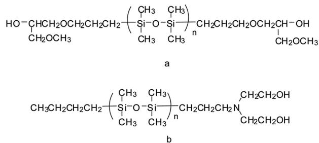
Fig. 1 Chemical structure of PDMS used to prepare block (a) and graft (b) PDMS-modified WPU.<sup>48</sup>
