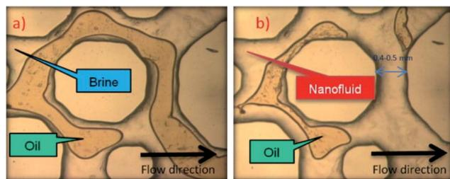
Fig. 4 Flooding experiment carried out with microfluidic chip (a) brine flooding (b) silica particle nanoflooding. Hendraningrat *et al.* concluded that nanofluid can potentially increase recovery rate. (Reprinted with permission from (ref. 48). Copyright (2013) Elsevier.)
