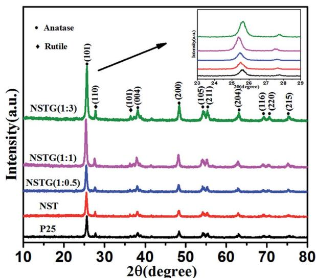
Fig. 1 XRD patterns of P25, NST, NSTG(1 : 0.5), NSTG(1 : 1), and NSTG(1 : 3). Inset XRD pattern shows the 23–29 degree region.
