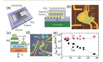
Fig. 3 Schematic illustration (a and c) and optical images (b and d) of the vertically stacked graphene/MoS2 heterostructured transistors. (e) The MoS<sub>2</sub> layer number dependence of the  $I_{on}$  (current density at  $V_{B}$  = +0.5 V and  $V_{\rm G}$  = +50 V) and  $I_{\rm off}$  (current density at  $V_{\rm B}$  = +0.5 V and  $V_{\rm G}$ = -50 V). Reprinted with permission from ref. 71 and 73. Copyright 2014 AIP Publishing LLC and 2013 Nature Publishing Group.
