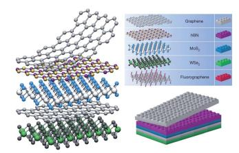
Fig. 2 Schematic 2D heterostructures based on van der Waals interlayer force. Reprinted with permission from ref. 67. Copyright 2013 Nature Publishing Group.
