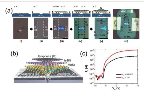
Fig. 5 (a) Schematics (not to scale) of the fabrication process steps (top) and the corresponding optical microscope images (bottom) of a representative graphene/BN/MoS<sub>2</sub> transistor. Scale bar is 5  $\mu$ m for all images. (b and c) Schematic illustration (b) and  $I_D - I_G$  characteristics at different  $V_G$  (c) of the graphene/BN/MoS<sub>2</sub> transistor. Reprinted with permission from ref. 75. Copyright 2015 ACS.
