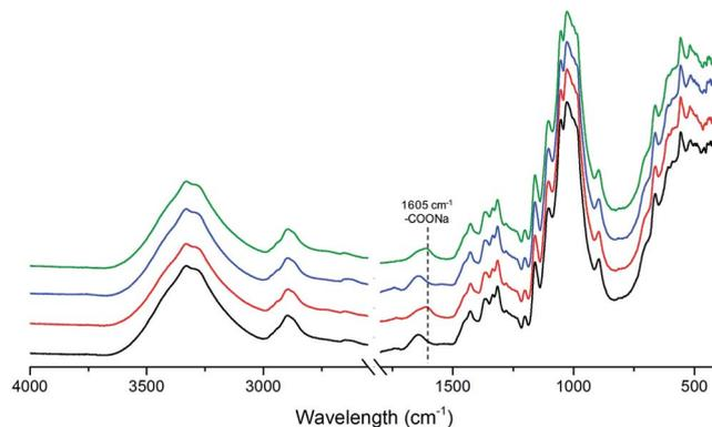
Fig. 2 FT-IR spectra of unmodified S/CNC<sub>BE</sub> (black curve), surface TEMPO oxidized S/CNC<sub>BE</sub> (red curve) and unmodified sludge (blue curve) membranes.
