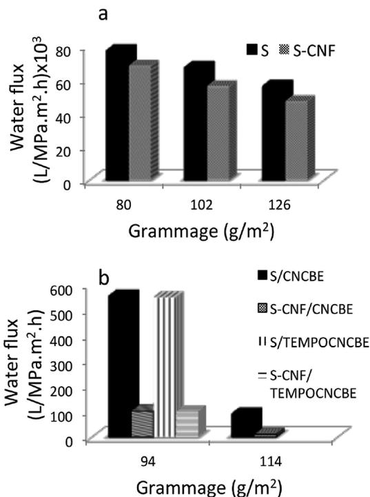
Fig. 6 Water flux of fabricated support layers with and without  $\text{CNF}_{\text{SL}}$  (a) with different grammage. Layered fabricated membranes indicate the decrease in water flux (b) but *in situ* TEMPO oxidation has no significant effect on water flux (b).
