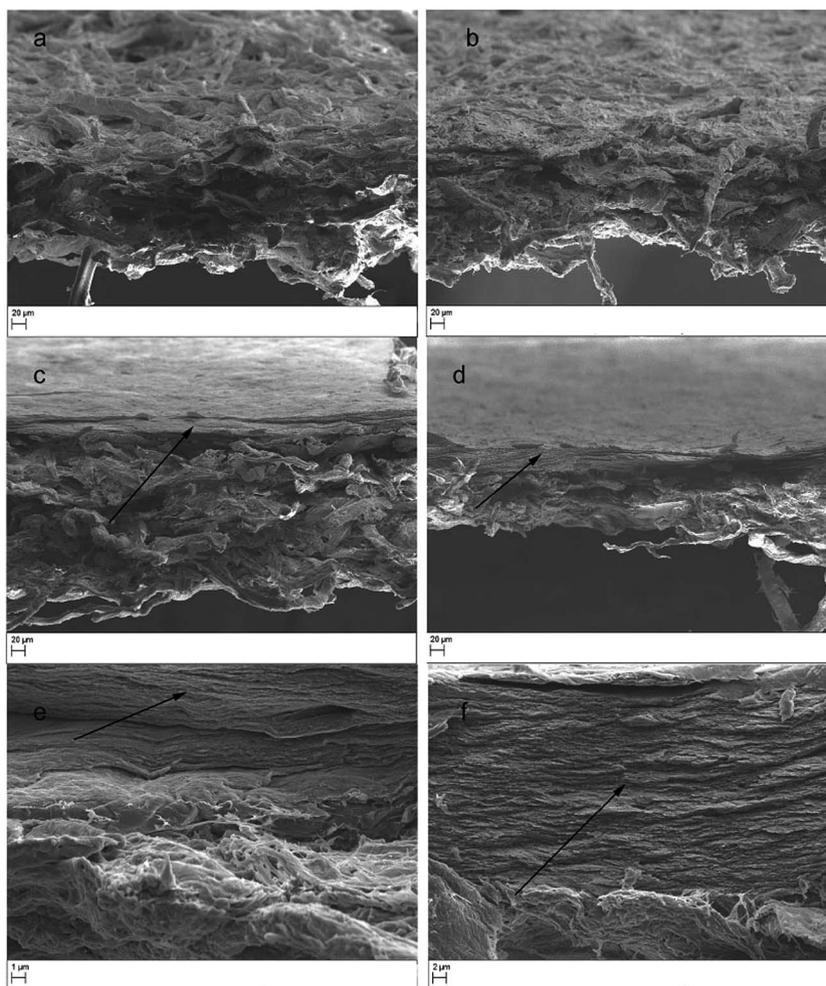
Fig. 3 SEM images of sludge (a) sludge–CNF<sub>SL</sub> (b) support layers. Bilayered membranes having S/CNC<sub>BE</sub> (c and e) and S–CNF<sub>SL</sub>/CNC<sub>BE</sub> (d and f) compositions with different resolutions were also shown. Layered structure of membranes is clearly visible having upper dense functional layer (as indicated by arrow) and lower loose network made up of sludge fibers or S–CNF<sub>SL</sub> mixture.
