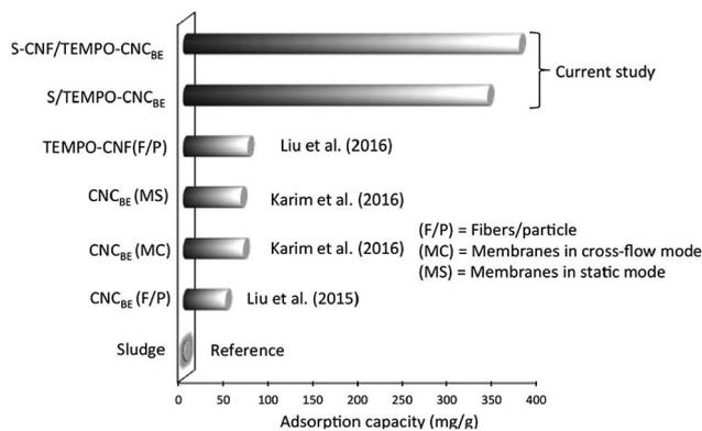
Fig. 7 A comparative study of adsorption capacity of Cu(II) with different operation parameters with two nanocellulose (CNF and CNC<sub>BE</sub>). Sludge was taken as reference in the current study. The highest adsorption capacity was recorded for *in situ* functionalized membranes as discussed in current study.
