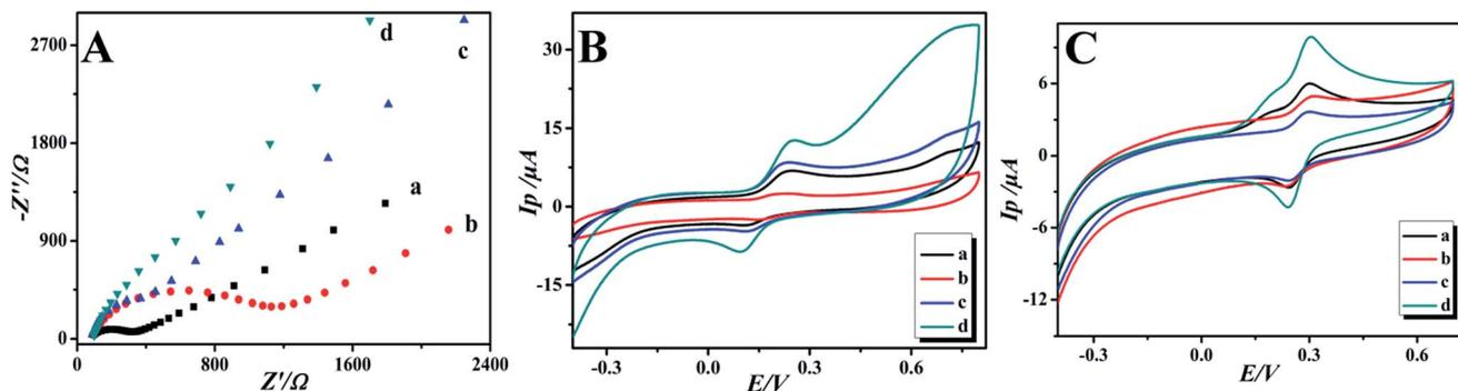
Fig. 3 Electrochemical impedance spectroscopy recorded in  $0.2 \text{ mM K}_3[\text{Fe}(\text{CN})_6]$  solution (A). Cyclic voltammograms showing the response of different modified electrodes to  $1 \mu\text{M}$  DA (B);  $1 \mu\text{M}$  DA and  $40 \mu\text{M}$  AA (C) in  $0.1 \text{ M PBS}$ . (a) GCE, (b) GO/GCE, (c) GO-IL/GCE, and (d) GO-IL-AuNPs/GCE.
