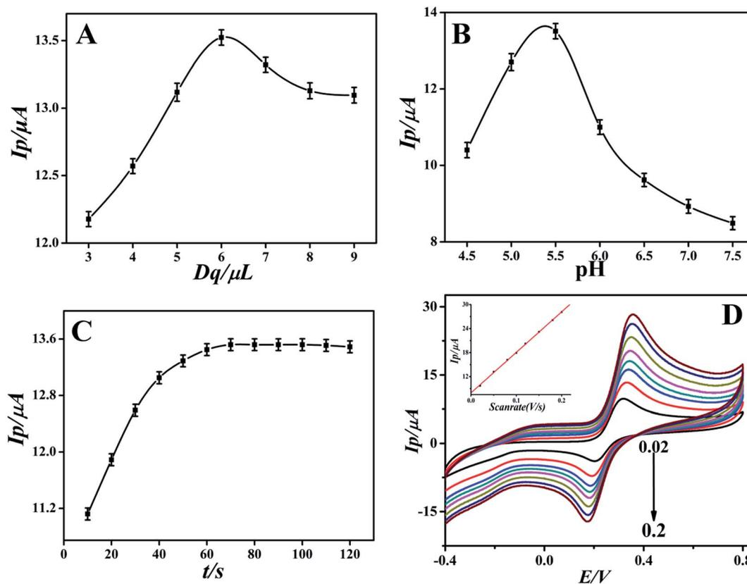
Fig. 4 (A) Effect of the volume of GO-IL-AuNPs. (B) Effect of pH value. (C) Effect of accumulation time. (D) CVs of GO-IL-AuNPs/GCE in 0.1 M PBS (pH 5.5) with 10  $\mu\text{M}$  DA at different scan rates (0.02, 0.05, 0.08, 0.1, 0.12, 0.15, 0.18, and 0.2  $\text{V s}^{-1}$ ). Inset: the linear relationship between peak current and scan rate.
