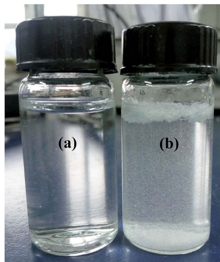
Fig. 7 The IBU solubilized by \beta -CDP (a) and its control group without the addition of \beta -CDP (b).
