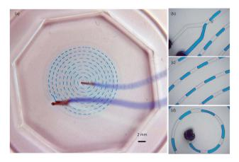
Fig. 8 Generation of blue dyed water droplets in corn oil with the spiral micro channel at a feed speed of 2 μL min<sup>-1</sup>, (a) global view, (b) pressure induced breaking of water in the inlet area, (c) spiral flow of the droplets, (d) outlet area.
