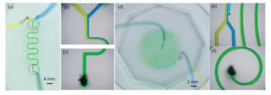
Fig. 7 3D printed micromixers mixing blue and yellow dyes (a) mixing in the winding microchannel at a feeding speed of  $10 \mu L \min^{-1}$ . Areas in the black circles are magnified in (b) and (c), (b) magnified inlet junction, (c) magnified fluid channel near the outlet, (d) mixing in the spiral microchannel at a feed speed of 100 µL min<sup>-1</sup>, (e) magnified spiral microchannel inlet junction, (f) magnified fluid channel near the spiral microchannel outlet.
