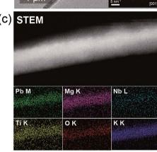
Fig. 2 (a) SEM image of PMN-PT NWs synthesized by a hydrothermal method. (b) TEM image of PMN-PT NWs. The Left-top inset is a HRTEM image of a single NW showing that lattice fringes of the (110) plane and the right-bottom image shows the SAED pattern when the electron beam is coherent along the [001] plane. (c) STEM image and EDS mapping of a PMN-PT NW.
