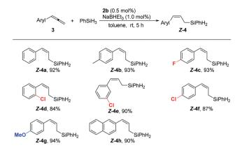
Scheme 2 Highly regio- and stereoselective hydrosilylation of aryl substituted allenes. The reaction was carried out with 1.0 mmol of 3, 1.0 mmol of PhSiH $_3$ , 5.0  $\mu$ mol of 2b, 10.0  $\mu$ mol of NaBHEt $_3$ , in 1 mL toluene at room temperature for 5 h. Yields of the isolated products are given.
