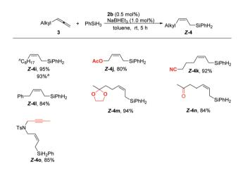
Scheme 3 Highly regio- and stereoselective hydrosilylation of alkyl substituted allenes. The reaction was carried out with 1.0 mmol of 3, 1.0 mmol of PhSiH $_3$ , 5.0  $\mu$ mol of 2b, 10.0  $\mu$ mol of NaBHEt $_3$ , in 1 mL toluene at room temperature for 5 h. Yields of the isolated products are given. <sup>a</sup> The reaction was carried out with 5 mmol of 3i to afford 1.2 g of Z-4i.
