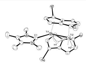
Fig. 3 ORTEP diagram of the molecular structure of (4) displaying 50% probability ellipsoids. Pr groups omitted for clarity
