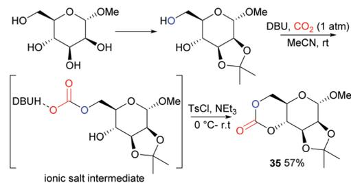
Fig. 21 Synthesis of *D*-mannose derived cyclic carbonate using CO<sub>2</sub> as a feedstock.
