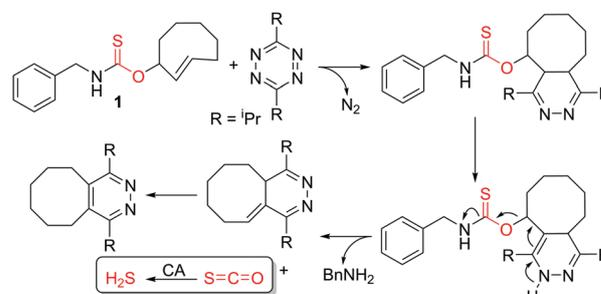
**Scheme 1** IEDDA reaction of thiocarbamate-functionalized TCO **1** with tetrazine to generate COS/H<sub>2</sub>S.
