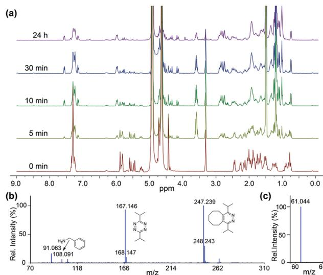
**Fig. 1** (a) <sup>1</sup>H NMR spectra of the reaction of **1** and tetrazine (b) ESI-MS of reaction products, confirming self-immolation. (c) MS confirmation of COS formation.
