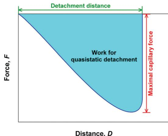
Fig. 3 Sketch of a force–distance curve for the process of particle retraction. From the  $F(D)$  curve, we can directly extract: the maximal (capillary) force  $F_{\max}$ , the detachment distance  $D_{\max}$  and the work for quasistatic detachment  $W$ .
