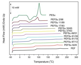
Fig. 3 DSC traces of guenched PEF, PESu and PEFSu copolymers.
