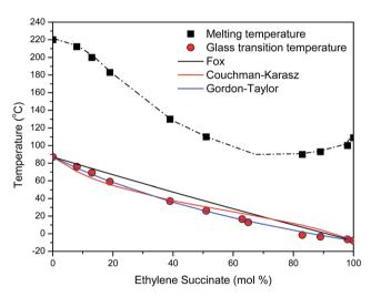
Fig. 4 Variation of the melting temperature  $(T_m)$  and glass transition temperature  $(T_q)$  of the PEFSu copolymers with composition.
