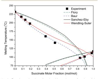
Fig. 8 Experimental and predicted melting point as a function of the succinate molar fraction.
