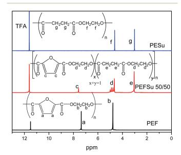
Fig. 1 Chemical structures and  $^1\mathrm{H}$  NMR spectra of PEF, PESu and the PEFSu 50/50 copolymer.
