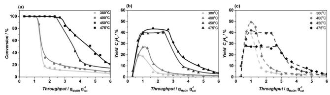
Fig. 5 Methanol conversion (a), yield of ethylene (b) and propylene at 380 °C ( $\blacksquare$ ,  $\blacktriangle$ ,  $\spadesuit$ ), 400 °C ( $\blacksquare$ ,  $\blacktriangle$ ,  $\spadesuit$ ) and 475 °C ( $\blacksquare$ ,  $\blacktriangle$ ,  $\spadesuit$ ) and 475 °C ( $\blacksquare$ ,  $\blacktriangle$ ,  $\spadesuit$ ) obtained in MTO reaction over Sigma1-315-M zeolite with SiO<sub>2</sub>/Al<sub>2</sub>O<sub>3</sub> = 315 and crystal size of 2.5 µm at standard operation conditions.
