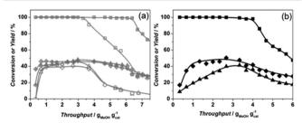
Fig. 8 Methanol conversion (■), ethylene (▲) and propylene (♦) yields of (a) Sigma1-315-S ( $\square$ ,  $\triangle$ ,  $\diamondsuit$ ) and Sigma1-315-S-m ( $\boxplus$ ,  $\triangle$ ,  $\diamondsuit$ ); (b) ZSM-58 ( $\blacksquare$ ,  $\blacktriangle$ ,  $\blacklozenge$ ) (SiO<sub>2</sub>/Al<sub>2</sub>O<sub>3</sub> = 110, 0.6–1.8  $\mu$ m) at 450 °C and standard operation conditions
