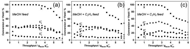
Fig. 9 Methanol conversion (■), ethylene (▲), propylene (♦) and butenes (●) yields obtained over Sigma1-315-S tested at 450 °C and standard operating conditions (a) 50% MeOH + 50%  $N_2$ ; (b) 45% MeOH + 10%  $C_2H_4$  + 45%  $N_2$ ; (c) 45% MeOH +10%  $C_3H_6$  + 45%  $N_2$ ; (c) 45% MeOH +10%  $N_2$  +10
