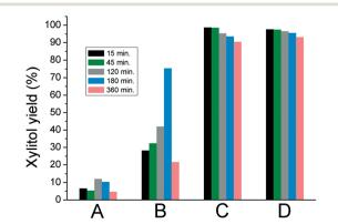
Fig. 3 Xylitol yield during different reaction times at 120 °C.
