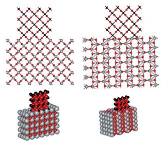
Fig. 6 Atomic structures of RuO2 on rutile (left) and anatase (right) TiO<sub>2</sub> showing the high degree of lattice matching of RuO<sub>2</sub> on rutile TiO<sub>2</sub> (created by viewerlite software).<sup>50</sup>
