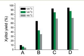
Fig. 1 Xylitol yield at different temperatures after 3 h reaction. Reaction conditions: 20 bar H<sub>2</sub>, xylose: Ru ratio 100:1 (w/w), solvent water.
