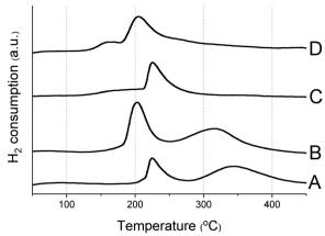
Fig. 4 TPR profiles for calcined Ru/TiO<sub>2</sub> catalysts.
