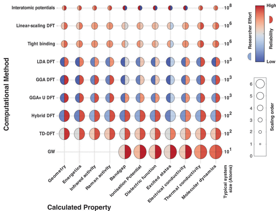
Fig. 2 Map showing the accessibility of different calculable material properties for a set of common computational methods. The methods include several flavours of density functional theory (DFT) which differ in the treatment of the quantum mechanical electron–electron interactions (e.g. local density approximation (LDA) and generalised gradient approximation (GGA)) as well as empirical tight-binding and many-body GW approaches. The circle size corresponds to the scaling of the computational effort with system size, the shading of the left semicircle represents the researcher effort required to use the method, and the shading of the right semicircle represents the reliability of the results from the method. Some properties are currently not calculable with GW theory for solids, and thus these circles are omitted.
