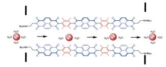
Fig. 27 Schematic representation of the NDI-based anion- $\pi$  slide for transmembranal anion transport.
