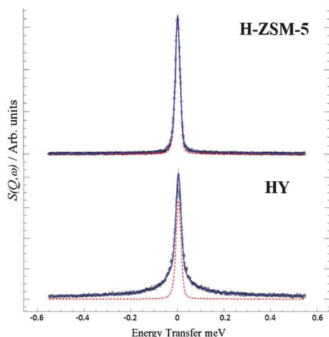
Fig. 1 QENS spectra obtained of methanol loaded in zeolites H-ZSM-5 and HY at  $Q = 0.9 \text{ \AA}^{-1}$  at 298 K, (---) represents the resolution data taken at 5 K. The close fit to the resolution function in H-ZSM-5 suggests immobilization, supporting framework methoxylation unlike the significant broadening in HY suggesting intact diffusing methanol.
