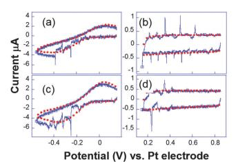
Fig. 9 Cyclic voltammograms recorded simultaneously ((a and c) and (b and d)) for two electrodes separated by 206  $\mu m$ . Conditions:  $K_3[Fe(CN)_6]$ (50 mM) in KNO<sub>3</sub> (0.1 M), horn-to-electrode distance 1 cm, electrode diameters 29  $\mu m$ . Voltammograms under silent conditions (red) and subject to 8.9 W cm<sup>-2</sup> insonation (blue) are represented. Adapted from ref. 67.
