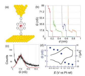
Fig. 4 (a) Schematization of a scanning tunneling microscopy break junction experiment. (b) A few conductance traces obtained for 1 at a sample potential of -0.3 V per Pt and a bias of 50 mV. Electrolyte: 0.1 M NaClO<sub>4</sub> aqueous solution. (c) Histogram obtained from the selection of 211 out of 1000 conductance traces. (d) Filled circles: molecular conductance versus sample potential. Black line: cyclic voltammogram. Adapted from ref. 45
