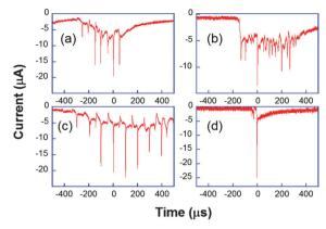
Fig. 8 Chronoamperometric current obtained for the reduction of K<sub>3</sub>[Fe(CN)<sub>6</sub>] (50 mM) in aqueous KNO<sub>3</sub> under ultrasound power of 8.9 W cm<sup>-2</sup> at a 29 μm diameter platinum electrode. Horn-to-electrode distances are 10 mm (a-c) and 1 cm (d). Adapted from ref. 67.
