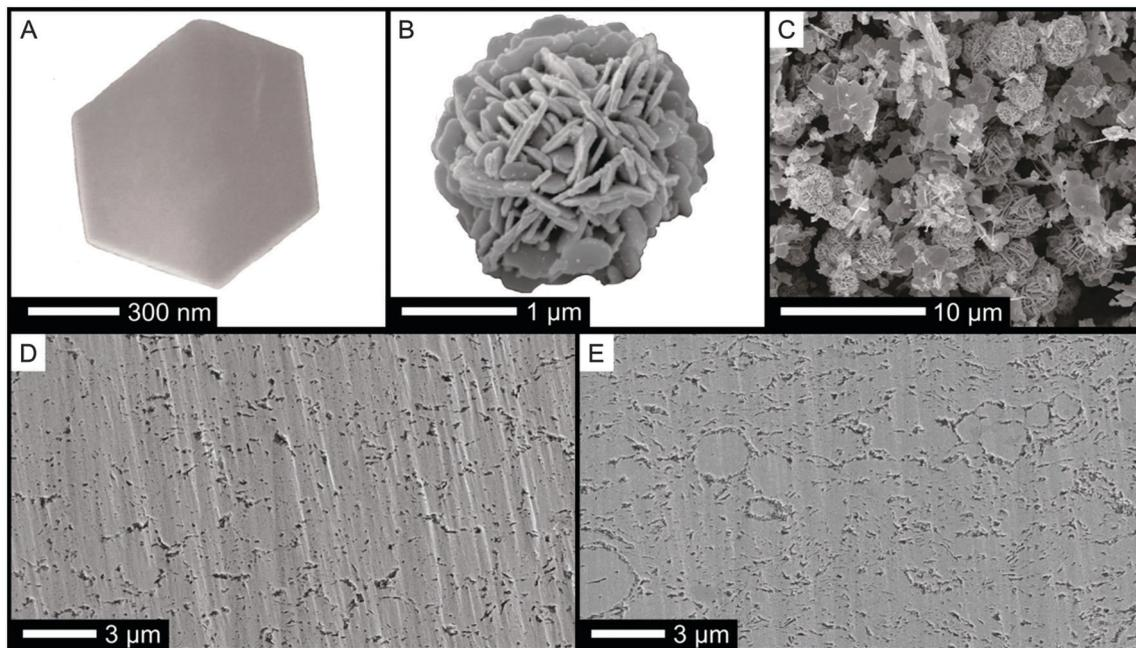
Fig. 2 SEM images of a single Sb<sub>2</sub>Te<sub>3</sub> nanoparticle (A), an isolated agglomerate (B) and the powder containing many of such agglomerates (C). Cross sections of two cold pressed pellets decomposed in the microwave for 5 min (sample I) with many agglomerates preserved within the microstructure (D) and in an oil bath for 4 h (sample II) showing only a few agglomerates in the microstructure (E).
