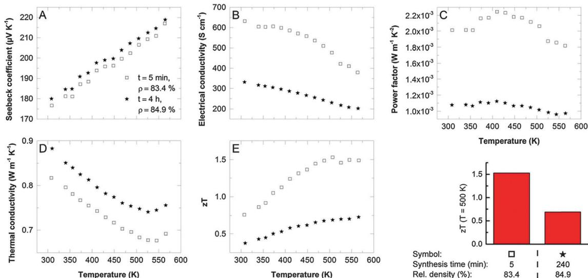
Fig. 3 Thermoelectric transport properties of two different  $\text{Sb}_2\text{Te}_3$  nanoporous bulk samples, synthesized at  $170^\circ\text{C}$  either within 5 minutes in IL using a microwave reactor (sample I,  $\square$ ) or within 4 hours by thermal decomposition in an oil bath (sample II,  $\star$ ).
