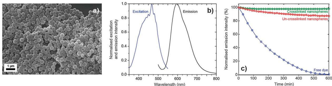
Fig. 2 (a) Representative SEM image showing fully formed and crosslinked nanospheres,  $\sim 300$  nm in diameter prepared from water. (b) Normalised photoluminescence excitation and emission spectra for the crosslinked nanospheres in water. (c) Normalised emission intensity versus time for crosslinked and non-crosslinked nanospheres in water under constant excitation at 450 nm. Also shown is equivalent data for the free dye in de-aerated ethanol.
