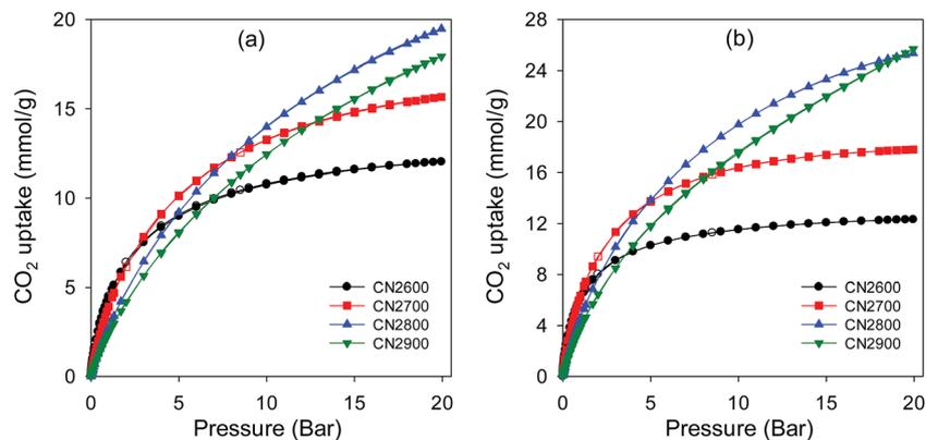
Fig. 9 CO<sub>2</sub> uptake isotherms at (a) 25 °C and (b) 0 °C in the pressure range 0–20 bar for activated CN2T carbons.
