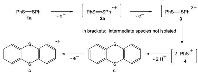
Scheme 1 Oxidation of diphenyldisulfide in conc. sulfuric acid.
