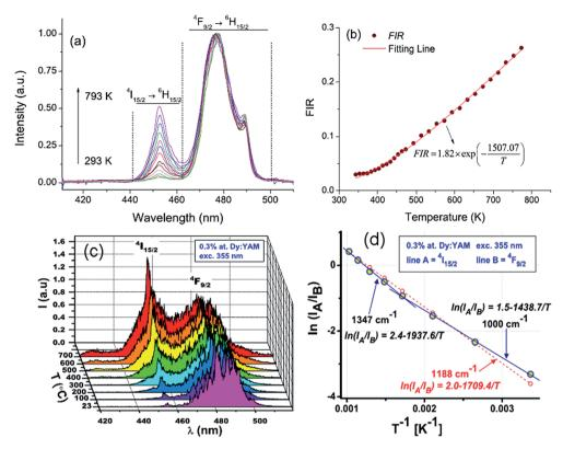
Fig. 16 Temperature dependent (a) emission spectra and (b) fluorescence intensity ratio (FIR) between the 455 nm and 478 nm emissions for the  $BaYF_5:2\%Dy^{3+}$  sample. Temperature dependent (c) emission spectra and (d) Arrhenius plot of the intensity ratio for  $Dy^{3+}$  doped  $Y_4Al_2O_9$  crystals. Reproduced from ref. 72 and 73 with permission of Optical Society of America and Elsevier.
