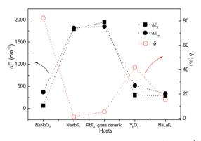
Fig. 8 Host dependent  $\Delta E_{\rm f}$  and  $\Delta E_{\rm m}$  between the TCL of Tm<sup>3+</sup> ions, and the corresponding  $\delta$  values.
