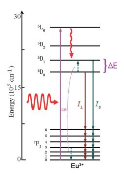
Fig. 17 The mechanism of optical thermal sensing through down-conversion of the  ${\rm Eu}^{3+}$  ion under infrared excitation.
