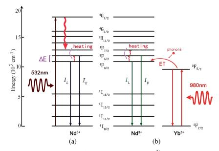
Fig. 12 The mechanism of optical thermal sensing through (1) down-conversion of the  $Nd^{3+}$  ion under 532 nm green excitation, and (2)  $Yb^{3+}$  –  $Nd^{3+}$  energy transfer under 980 nm infrared excitation.
