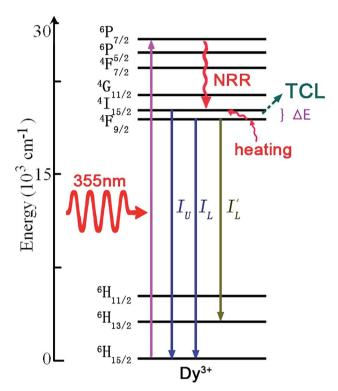
Fig. 15 The mechanism of optical thermal sensing through down-conversion of the  ${\rm Dy}^{3+}$  ion under 355 nm ultraviolet excitation.
