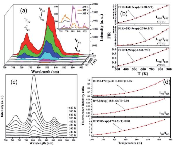
Fig. 13 Temperature dependent (a) near infrared emission spectra and (b) fluorescence intensity ratio (FIR) in  $Nd^{3+}/Yb^{3+}$  co-doped CaWO<sub>4</sub> phosphors excited by a 980 nm laser. Temperature dependent (c) near infrared emission spectra and (d) FIR in  $Nd^{3+}/Yb^{3+}$  co-doped oxyfluoride glass ceramic containing PbF<sub>2</sub> nanocrystals excited by a 980 nm laser. Reproduced from ref. 70 and 71 with permission of Optical Society of America and Elsevier.
