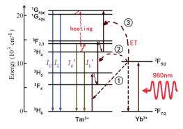
Fig. 6 The mechanism of optical thermal sensing through Yb<sup>3+</sup>-Tm<sup>3+</sup> energy transfer under 980 nm infrared excitation.
