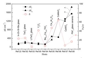
Fig. 11 Host dependent  $\Delta E_{\rm f}$  and  $\Delta E_{\rm m}$  between the TCL of Ho<sup>3+</sup> ions, and the corresponding  $\delta$  values.
