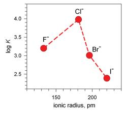
Fig. 12 Selectivity pattern for the affinity of halides towards the dimetallic cryptate receptor  $[Cu_2^{II}(3)]^{4+}$ . Log K values refer to the equilibrium:  $[Cu_{2}^{II}(3)]^{4+} + X^{-} \rightleftharpoons [Cu_{2}^{II}(3)(X)]^{3+}$  at pH = 5.25;  $(X^{-} = halide anion).^{20}$
