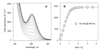
Fig. 5 (a) Spectra obtained over the course of the titration with  $\text{NaN}_3$  of an aqueous solution containing  $\text{Cu}(\text{CF}_3\text{SO}_3)_2$  and 7 in a 2:1 molar ratio, buffered at pH 8, at 25 °C; (b) titration profile (molar absorbance at 400 nm vs. equiv. of  $\text{NaN}_3$ ), indicating the formation of a 1:1 receptoranion complex.<sup>14</sup>
