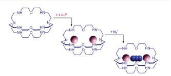
Fig. 1 Cascade process for the consecutive inclusion of two Cu<sup>II</sup> ions, then of one azide anion into the bistren cryptand 2, to form the ternary dimetallic complex  $[Cu_2^{11}(2)(N_3)]^{3+}$ . Each terminal atom of the ambidentate anion establishes a coordinative interaction with a coordinatively unsaturated Cu<sup>II</sup> centre bound to each tren subunit.
