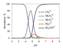
Fig. 4 Concentration profiles (%) of the species present at the equilibrium over the 2-9 pH range, for a solution  $10^{-3}$  M in 7 and  $2 \times 10^{-3}$  M in  $Cu^{II}$ , calculated from the log K values reported in ref. 13 L = 7.
