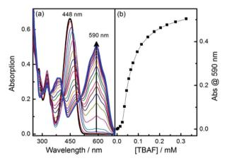
Fig. 2 (a) Absorption spectra changes of probe 1 along with addition of fluoride anion in MeCN; (b) Plot of absorption at 590 nm *versus* concentration of TBAF [1] =  $10 \mu M$ .
