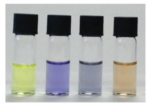
Fig. 4 Colour changes of probe 1 after treatment with different anions. Samples show, from left to right: 12 uM probe 1, 13 equiv. of each anions or the anions  $F^-$ ,  $OAc^-$ ,  $H_2PO_4^-$  respectively.
