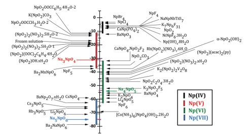
Fig. 6 Isomer shifts versus NpAl<sub>2</sub> of Np(IV), Np(VI), Np(VI), and Np(VII) compounds after (ref. 22). The present result for Na<sub>3</sub>NpO<sub>4</sub> is shown in red together with Na<sub>4</sub>NpO<sub>5</sub> (green) and Na<sub>5</sub>NpO<sub>6</sub> (blue) reported in (ref. 11).
