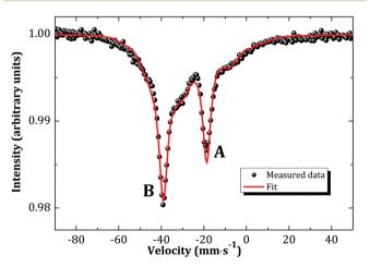
Fig. 7 Mössbauer spectrum of the cubic phase "X" recorded at 4.2 K and fitted to the model (see text).
