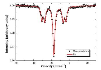
Fig. 5 Mössbauer spectrum of  $\alpha$ -Na<sub>3</sub>NpO<sub>4</sub> recorded at 4.2 K and fitted to the model (see text).
