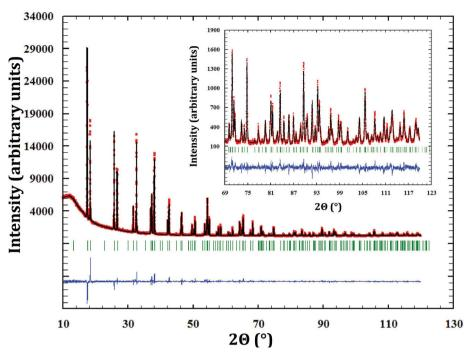
Fig. 1 Comparison between the observed ( $Y_{obs}$ , in red) and calculated ( $Y_{calc}$ , in black) X-ray diffraction patterns of  $\alpha$ -Na<sub>3</sub>NpO<sub>4</sub>.  $Y_{obs} - Y_{calc}$ , in blue is the difference between the experimental and calculated intensities. The Bragg reflections are marked in green. Measurement at  $\lambda$  = Cu-K $\alpha$ 1.
