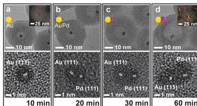
Fig. 2 TEM (upper) and HRTEM (lower) images of samples isolated during the reaction of the  $(\text{Fe}_3\text{O}_4/\text{Au})@(\text{SiO}_2/\text{Pd}^{2+})$  with  $\text{NaBH}_4$  at (a) 10, (b) 20, (c) 30, and (d) 60 min, respectively. Insets: EDX elementary maps for showing the distribution of Au (red) and Pd (yellow) elements.
