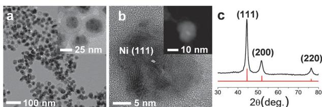
Fig. 3 (a) TEM, (b) HRTEM and STEM-HAADF (inset) images and (c) XRD pattern of the  $\text{Ni}@h\text{-SiO}_2$ . The red line in (c) shows the position of the reflections corresponding to the fcc Ni phase (JCPDS Card No. 01-1260).
