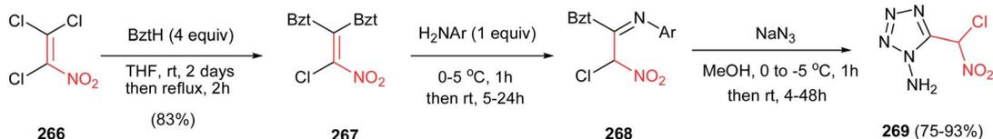
Scheme 89 Synthesis of tetrazoles starting with 1,1,2-trichloro-2-nitroethene.
