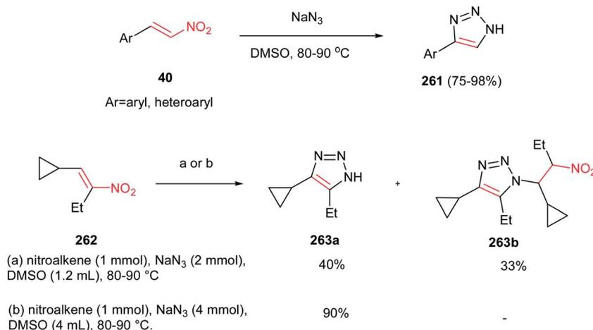
Scheme 87 Catalyst-free synthesis of triazoles from nitroalkenes and NaN<sub>3</sub>.
