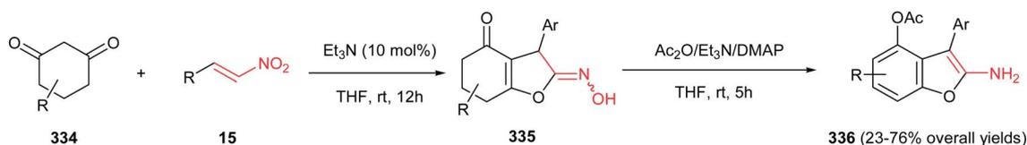
Scheme 114 Formation of 4-acetoxy-2-amino-3-arylbenzofurans from 1-aryl-2-nitroethylenes and cyclohexane-1,3-diones.
