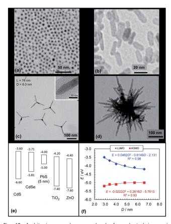
Fig. 10 Architectures and energy levels for selected inorganic acceptors. TEM images of PbS NCs (a), ZnO NRs (b), CdSe tetrapods (c) and hyperbranched CdSe (d). (e) Energy levels for various NCs. The energy levels for CdS, CdSe, PbS,  $TiO_2$  and ZnO were obtained from ref. 62, 155, 165, 166 and 167. (f) Size dependence of PbS NC energy levels plotted from the data reported in ref. 165. Figures reproduced with permission from: (b) ref. 168, (c) ref. 163 and (d) ref. 164.
