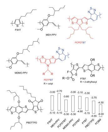
Fig. 7 Structures and energy levels for selected polymer donors. The energy levels for P3HT are taken from ref. 45 and 46. The energy levels for MEH-PPV, PCPDTBT, MDMO-PPV, PDTPBT, PTB7 and PBDTTPD are taken from ref. 62, 63, 64, 65, 41 and 66. The energy levels for PCBM are shown for comparison and are from ref. 45. The red and blue units are the donor and acceptor units, respectively
