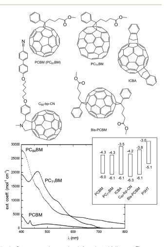
Fig. 8 Structures and energy levels for selected fullerenes. The energy levels for PCBM, PC71BM, ICBA, C60-bp-CN and bis-PCBM are from ref. 45, 52 and 75, 76 and 77, respectively. The energy levels for P3HT are shown for comparison. The UV-visible spectrum is reproduced with permission from ref. 73.
