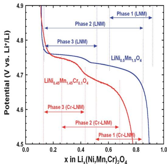
Fig. 15 Variation of the voltage as a function of the Li concentration  $x$  in un-doped and Cr-doped LNM samples during the discharge of cells cycled at  $C/24$  rate in relation to the phase diagram. Reproduced with permission.<sup>77</sup>
