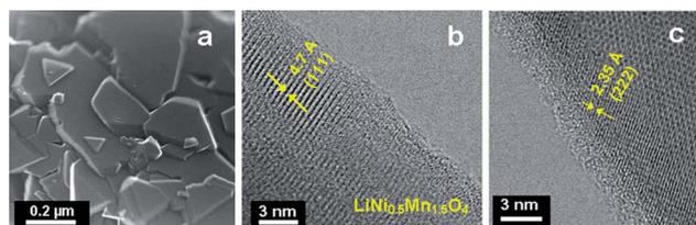
Fig. 2 SEM and TEM images of the LNM particles synthesized by co-precipitation.
