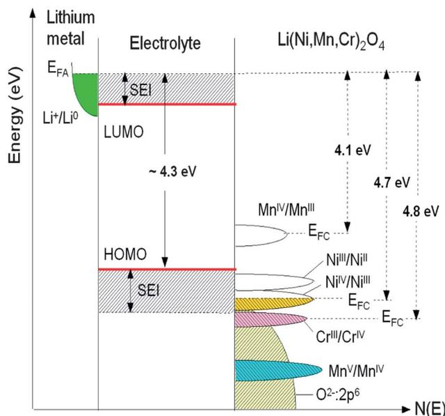
Fig. 7 Schematic density of states and Fermi energies for  $\text{Li}_x\text{Ni}_{0.5-y}\text{Mn}_{1.5-y}\text{Cr}_{2y}\text{O}_4$  spinel cathode. The Li permeable SEI layer formed on the electrode surface preserves the overall reversible reaction.
