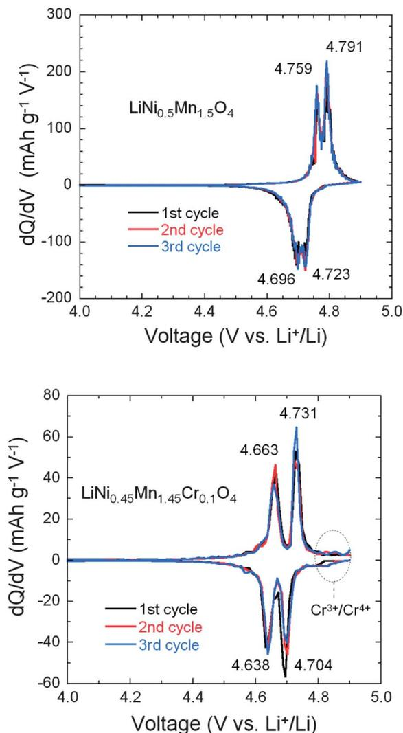
Fig. 11 Differential capacity curves,  $dQ/dV$  vs.  $V$ , of the un-doped LNM (top) and  $\text{LiNi}_{0.45}\text{Mn}_{1.45}\text{Cr}_{0.1}\text{O}_4$  (bottom). The values at the peaks are given in volt. Reproduced with permission.<sup>64</sup>
