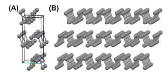
Fig. 1 The chemical structures of the compounds in this study. (A) The orthorhombic unit cell of black phosphorus  $^{19}$  (a = 3.31 Å, b = 4.38 Å c =10.50 Å,  $\alpha = \beta = \gamma = 90^{\circ}$ ; space group *Bmab*; Crystallography Open Database ID: 1010325) which generates a layer structure comprising corrugated lamellae of phosphorus atoms held together by weak interlayer forces. (B) Three-layer phosphorene.
