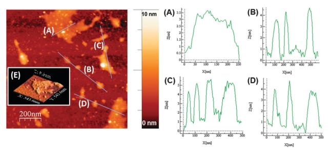
Fig. 3 Atomic force microscopy height profile image of few-layer phosphorene sheets produced from ultrasonic exfoliation of bulk phosphorus in NMP for 24 h and spin-coated onto a  $SiO_2/Si$  substrate. (A), (B), (C) and (D) show z-profiles of phosphorene flakes (N = 11) along the lines marked in the AFM relief image. Inset: (E) three-dimensional representation of the large ca. three-layer phosphorene flake observed at point (A)
